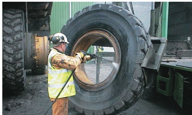
Cleaning the tire, 1 st step in demounting
