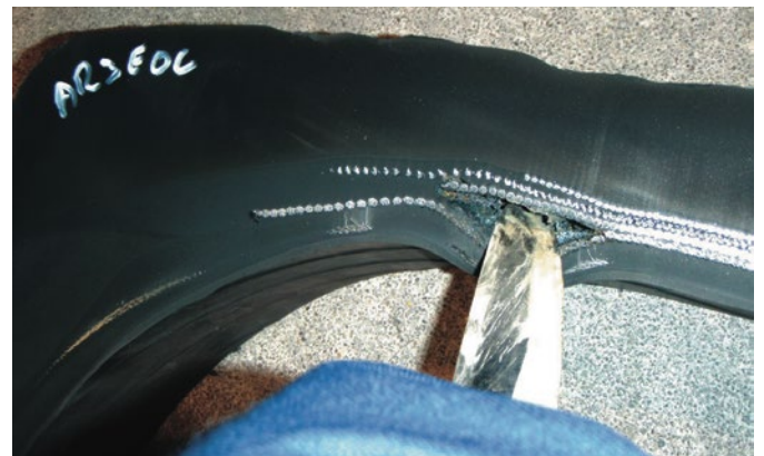
Separation of the components in a tire
