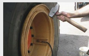
12 Inflate and lightly tap the locking ring
